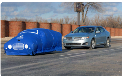
Adaptive cruise control and collision warning with brake support balloon-testing on Lincoln MKS.
