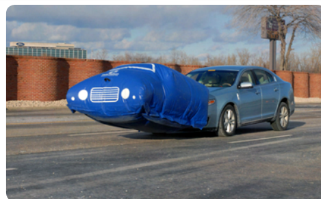
Adaptive cruise control and collision warning with brake support balloon-testing on Lincoln MKS.
