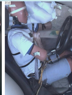
Adaptive vent blocked for larger occupant.
