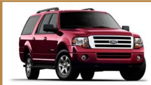
Expedition EL is unique from the B-pillar back with its own floor pan, one-piece bodyside, running boards, fascia, roof rack, rear quarter glass, one-piece headliner and quarter panel trim. The second-row doors are also unique, providing better ingress and egress to both the second and third rows.
