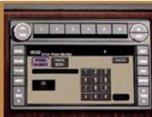
HomeLink gives the vehicle the technology to learn up to three garage door and power gate remote control codes, eliminating the need to clutter the interior with separate remote control units.
