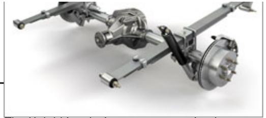
*The Hotchkiss-design rear suspension has been optimized with shock absorbers placed outboard of the frame rails to provide a smoother ride. Specifically, the design improves control of body lean, along with axle "skipping" and "skating" that can happen on washboard-type surfaces.*
