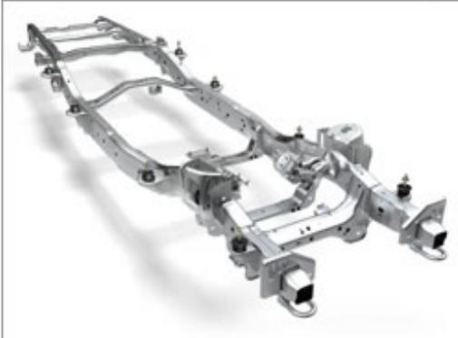
The fully boxed frame with hydroformed front rails is about nine times stiffer in torsion and approximately 50 percent stiffer in bending compared to the previous generation Ford F-150. The result is less shakes and shudders on rough roads.
