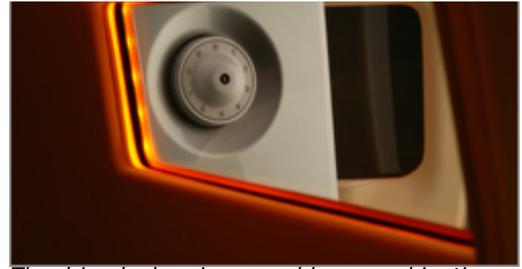
*The driver's door is opened by a combination lock.*
