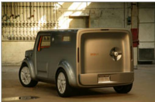
*The rear hatch is six inches thick, and features beveled edges like a bank vault.*
