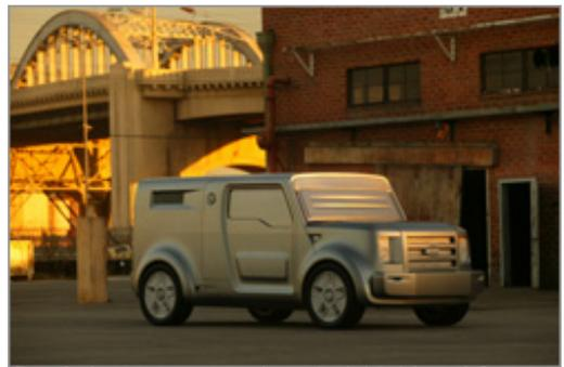
*Steel shutters cover the windshield and front windows, while the rear side windows are made of bullet-resistant glass.*
