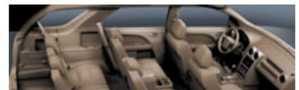
capability. When bucket seats are selected, second-row seats on limited models are mounted on optional adjustable tracks to increase legroom.
