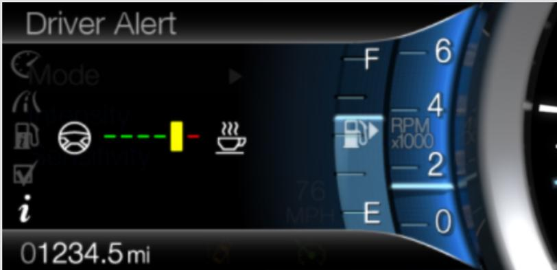
The Driver Alert System is designed to help alert drowsy drivers by monitoring the vehicle's movement compared to lane markings that are tracked by a camera mounted on the windshield. If the system detects a driving pattern consistent with a drowsy driver, a first-level chime will sound and a coffee cup warning will appear on the dashboard instrument cluster to recommend the driver take a break.
