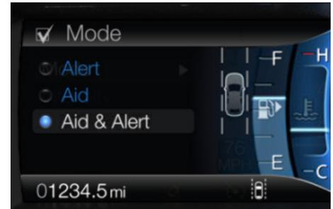
Lane assist is accessed in the left-hand cluster display using the left-hand five-way steering wheel switch.
