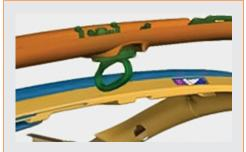
A new one-handed center latch lets the driver release the power-top without leaning across the car.
