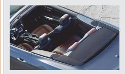
Simple snap-in side caps complete the clean top-down appearance and stow easily in the trunk.
