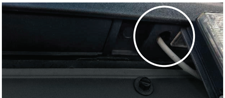
Close up of after-market light and wiring.
