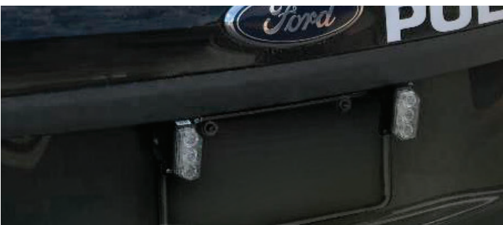
Police Interceptor Utility with after-market lights installed.
