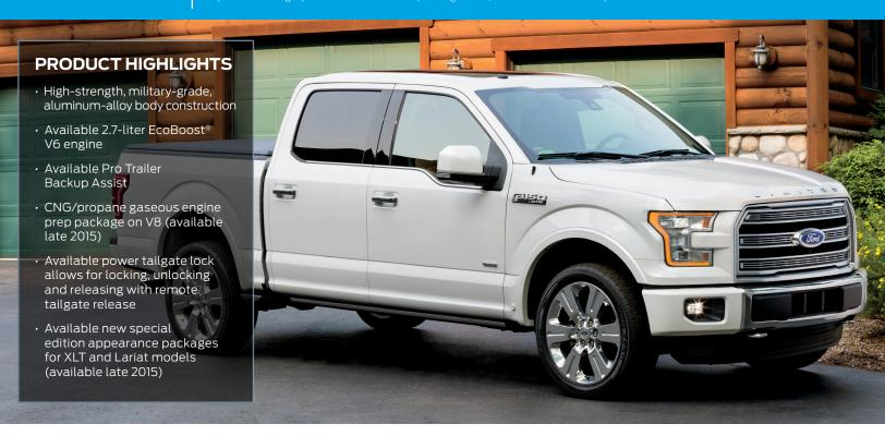
Engines: 2.7-liter EcoBoost 4x2, 325 horsepower, 375 lb.-ft. torque; maximum towing, 8,500 pounds, maximum payload, 2,250 pounds; EPA-estimated 19 mpg city, 26 mpg highway, 22 mpg combined
