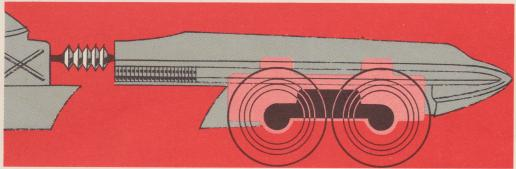
The entire front end of Seattle-ite XXI would uncouple from the passenger compartment and an optional power unit could be quickly installed. All controls would be conducted through a flexible coupling (Fig. 1) that would simply plug into the passenger compartment.
