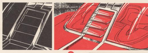
Jalousie windows (Fig. 5) could improve ventilation and reduce noise. At left is a close-up view of the windows in a closed position; at right they are open.
