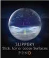
**Slippery** offers maximum stability control and reduces the amount of power going to the wheels with a less aggressive pedal response.
