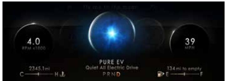
**Pure EV** is designed to keep the driver in all-electric mode in most conditions; should demand exceed electric capacity, the driver will receive a prompt to allow the gas engine to engage. All systems are set for maximum efficiency and a quiet, all-electric drive experience.
