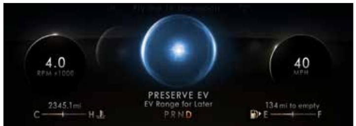
**Preserve EV** recharges and saves battery power for a later time, while continuing to use both the engine and motor to deliver the full performance our clients expect. The battery can be recharged up to about 75 percent state of charge when in this mode.
