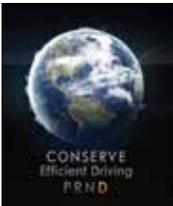
**Conserve** is an efficiency mode; the pedal response is less aggressive, while vehicle performance is tuned to optimize fuel efficiency.
