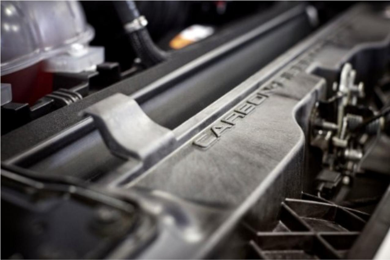
Weight balance is essential for high-performance cornering and braking – both on and off the track. When weight can be removed from the nose, the benefit is drastic. Ford Performance engineers created a forged carbon fiber grille opening reinforcement for Shelby GT350 that is roughly 24 percent lighter than an equivalent stamped-steel component. The reduction of weight in the nose of the car allows for enhanced balance and more predictable handling.
